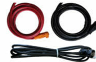
Model: AI-W5.1-PCable Details: Pair of 2/0AWG DC power cable and RJ45 communication cable connect with hybrid inverter, one end has a waterproof terminal . The cable length can be customized based on customer requirements, default length is 1500mm.
