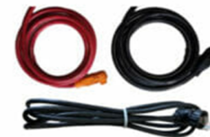
Model: AI-W5.1-BCable Details: Pair of 2/0AWG DC power cable and RJ45 communication cable for external battery expansion, power cable one end has a waterproof terminal, communication cable both ends have waterproof terminals . The cable length can be customized based on customer requirements, default length is 1500mm.
